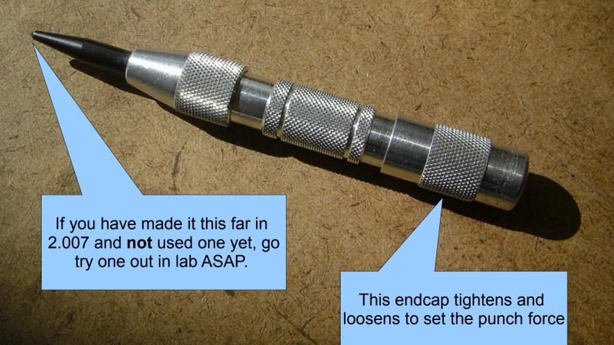
Make a dimple with the center punch, aligning the point with the intersection of your two lines.
