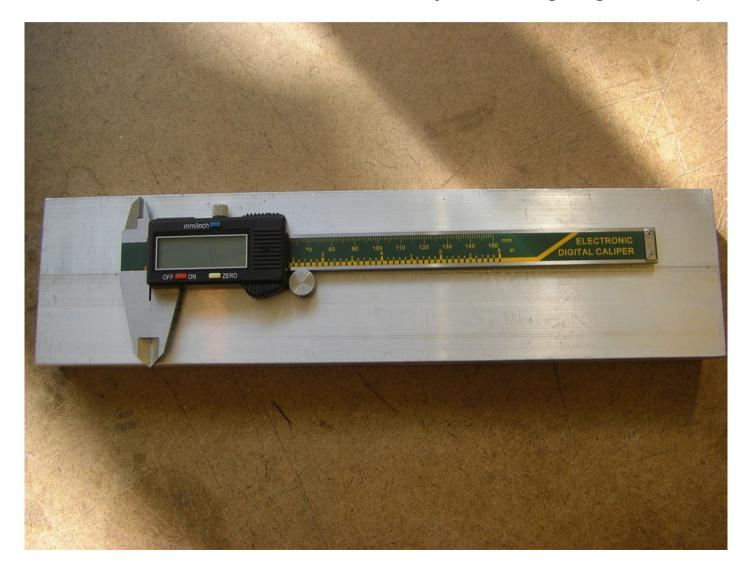
In your 2.007 kit, you have been provided with a set of 6" (150mm) digital calipers. You should use these not only for measuring and ascertaining dimensions of parts, but for accurate positioning of holes and other features when manually fabricating a part.
