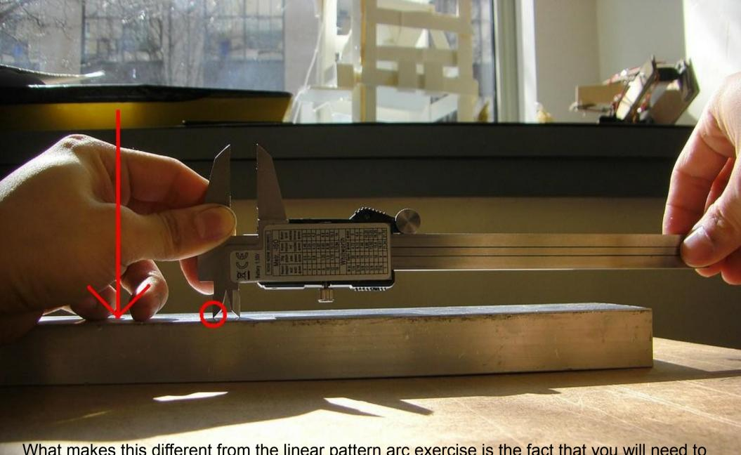
What makes this different from the linear pattern arc exercise is the fact that you will need to mark at different angular positions. For maximum control, keep one hand on the reference tip and make sure there is pressure on *it* at all times.
